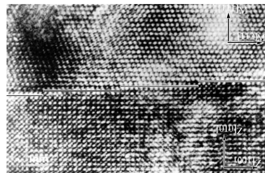
Fig. 9. High-resolution electron micrograph of the lamellar interface observed in the directionally solidified \text{MgO} - \text{ZrO}_2 eutectic.
